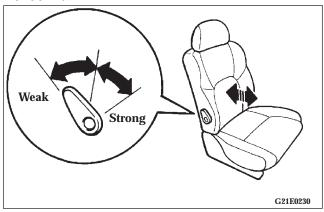
A lumbar support is included in the seatback of the driver's seat. The support has a three position adjustment.
